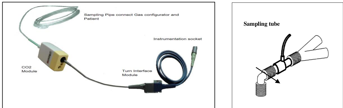
Figure 14-4 ISA™ Sidestream Analyzer (ISA CO 2 ) CO 2 Connection Schematic
