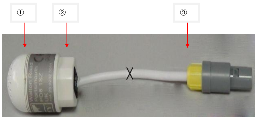
Figure 16-1 Connecting Oxygen Sensor
